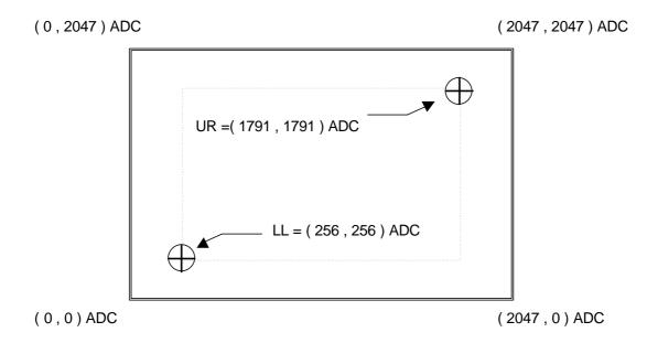
LL and UR are the calibration target points of touch panel, the points are setup at
